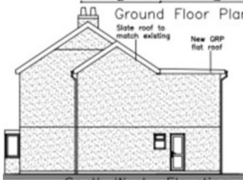
South West Elevation
